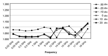
Figure 1. Typical SWR for the E9321A and E9325A sensors at various power levels
