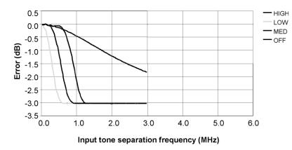
Figure 6. E9321A and E9325A Error in peak-to-average measurements for a two-tone input (high, medium, low and off filters).
